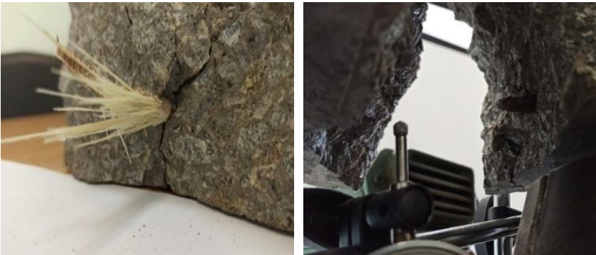
Fig. 3. Appearance of broken reinforcement d=8 mm in the samples after the test
