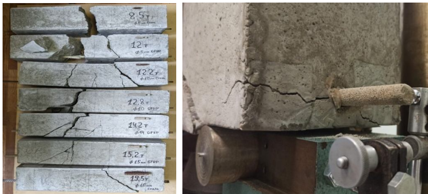
Fig. 4. Samples after testing
